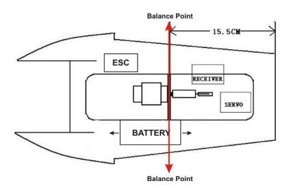
Adjust the battery fore and aft to obtain the balance point shown at 15.5cm – 6.1" from the stern of the boat.
